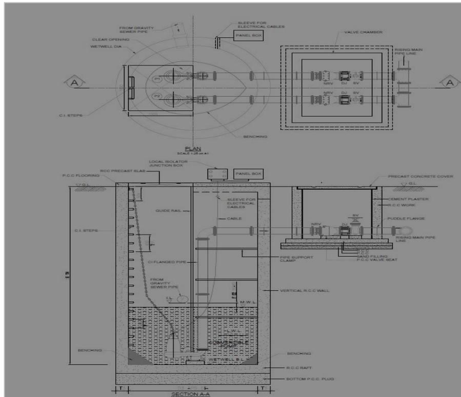
**Figure 6 Typical Lift station arrangement**
